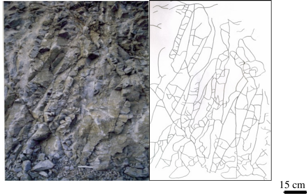
(d) Outcrop: A producing formation (marble) in Field 1 (photo and fracture trace map).
