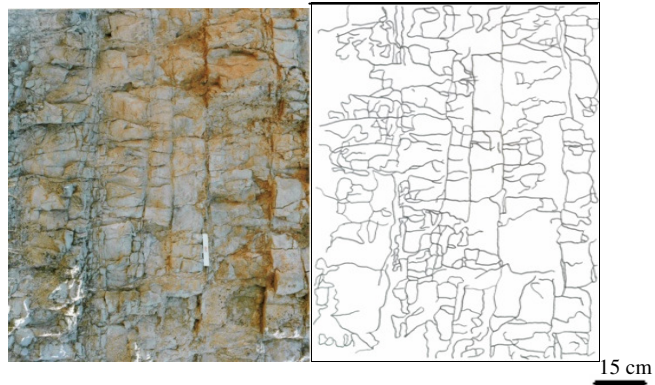
(a) Outcrop: A producing formation (limestone) in Field 5 lower formation (photo and fracture trace map).
